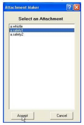
Click on an attachment and press the "Accept" button to select. "Cancel" turns off the selection window. Remember that the selected attachment is yellow on the drawing.
